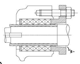
Shield grids being removed during installation of the gland packing, it must be ensured that they are replaced as soon as this operation is completed.
